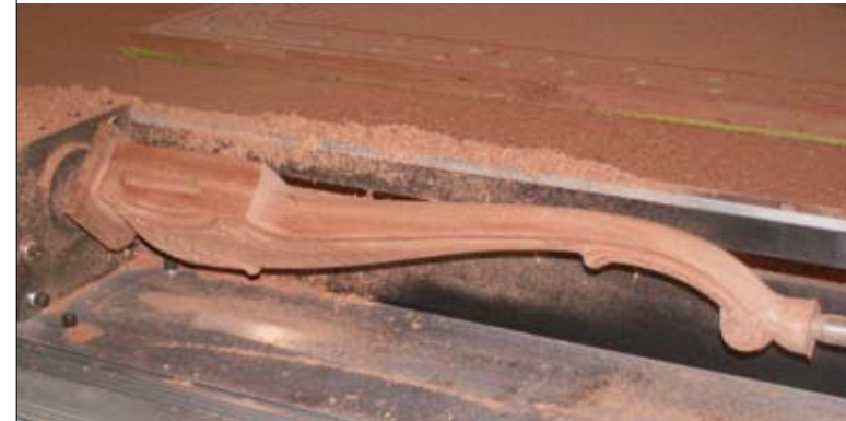
Legs being machined using the rotary playback
